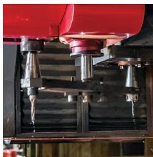
Quick 2-second spindle tool change for less downtime than manual processing
