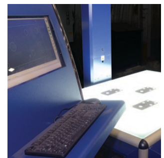
Inspection Planar provides inspection and reverse engineering of flat parts
